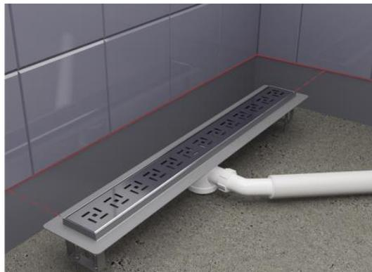
2. Connect the channel to the drainage system and set the height using the adjustable legs so that the upper edge of the frame is approximately 1mm below the
